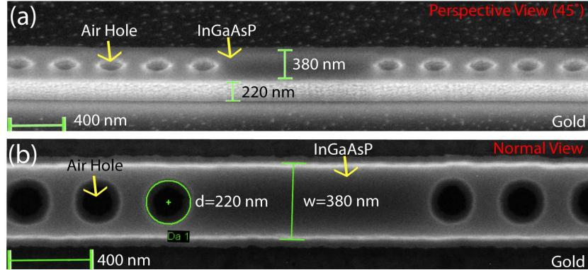
Fig. 2: Scanning electron micrographs of (a) a perspective view and (b) a surface normal view of the final fabricated structure are shown. The final device dimensions are also noted along with scale bars. A semiconductor layer is patterned on a gold film.
